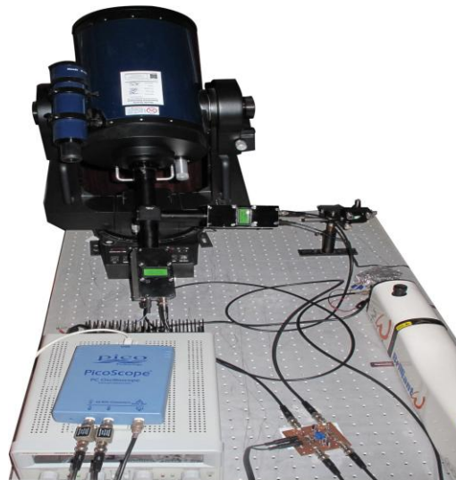
LIDAR system developed at IOP, VAST for investigating physical properties of atmosphere.
