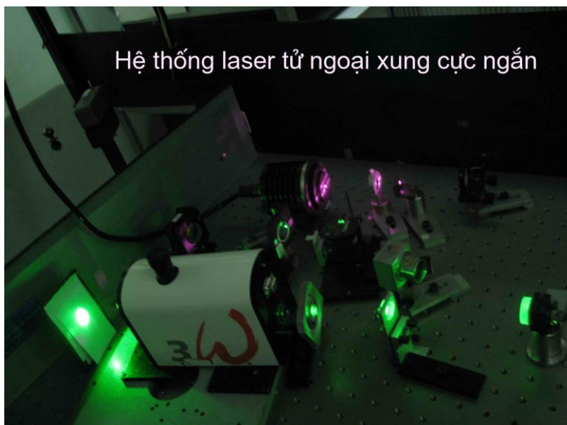
IR, VIS and UV picosecond laser developed at IOP, VAST
