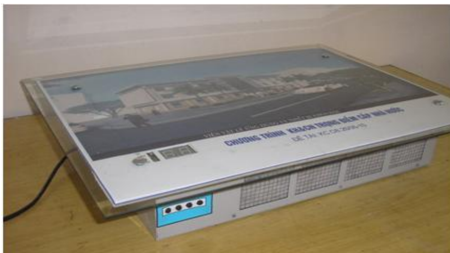
Device of cleaning the air on TiO_2 photocatalytic principle
